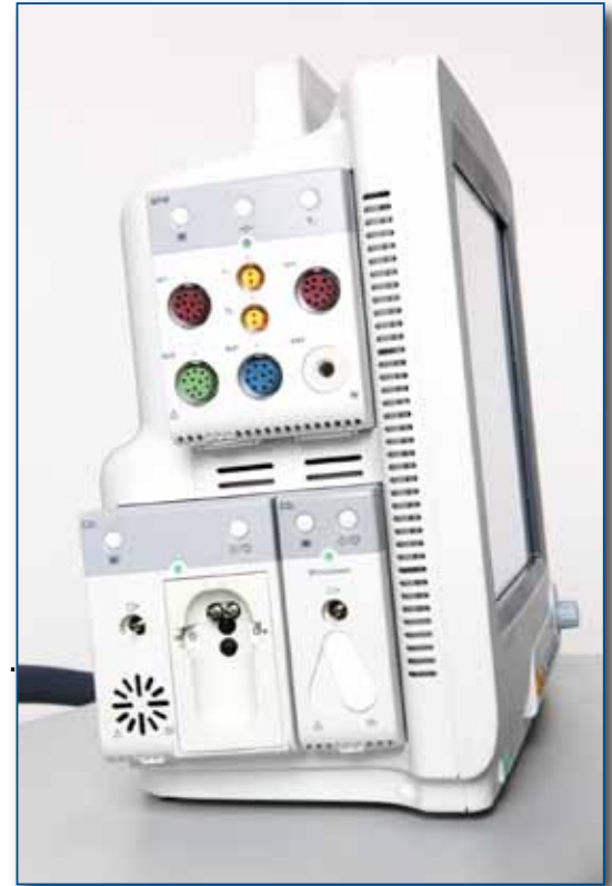
STANDARD INTEGRATED 5 SLOTS SUPPORTS UP TO 13 SLOTS WITH EXTERNAL SATELLITE MODULE RACK (OPTIONAL)
